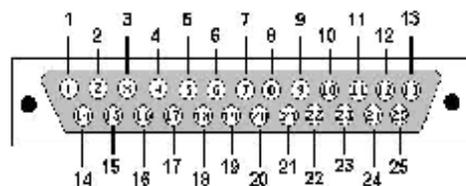
Diagram showing the pinout for the 25-way D-type connector.
